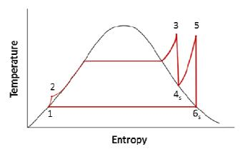
Figure 3.4.2b: T-s diagram for the Rankine cycle with reheat (subcritical)
