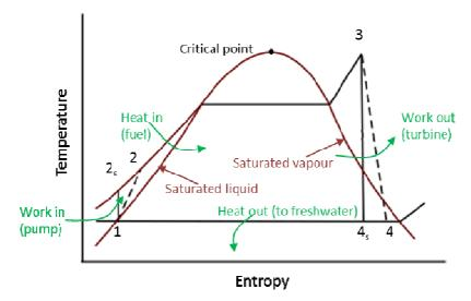
Figure 3.4.2a T-s diagram for the Rankine cycle (subcritical).
