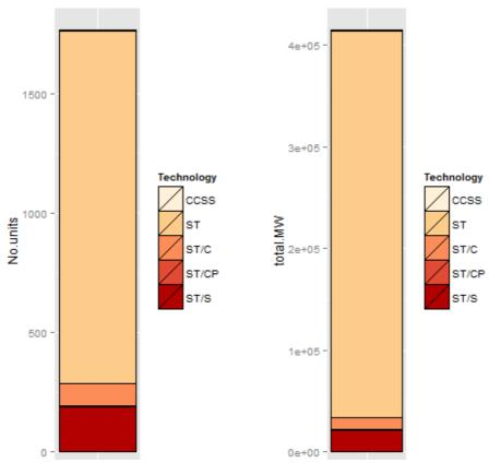
Figure 3.4.1: Left: number of units of thermal power stations per specific technology; Right: total gross electrical generating capacity per specific technology of thermal power station.
