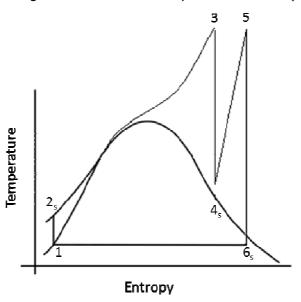
Figure 3.4.2c: T-s diagram for the Rankine cycle with reheat (supercritical)
