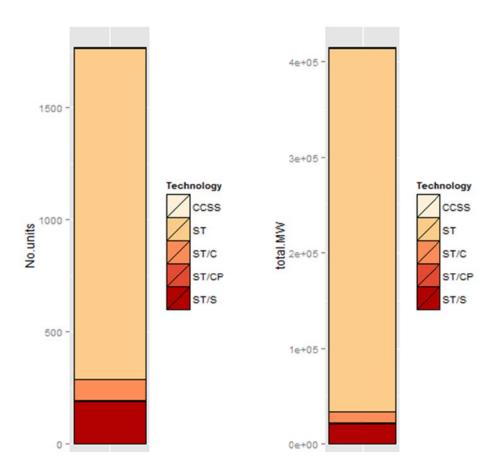
**Figure 4.1.1** Left: number of units of thermal power stations per specific technology; Right: total gross electrical generating capacity per specific technology of thermal power station.
