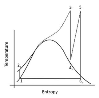
Figure 4.1.2c T-s diagram for the Rankine cycle with reheat (supercritical)
