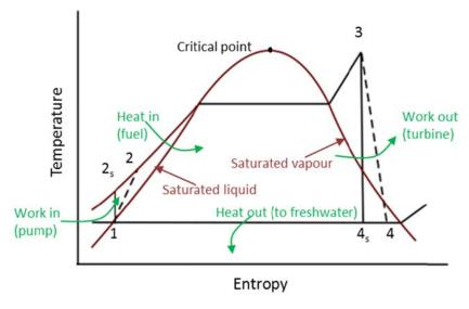
Figure 4.1.2a T-s diagram for the Rankine cycle (subcritical).
