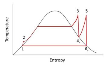
Figure 4.1.2b T-s diagram for the Rankine cycle with reheat (subcritical)
