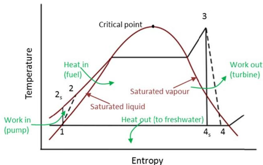
**Figure 4.1.2a** T-s diagram for the Rankine cycle (subcritical).
